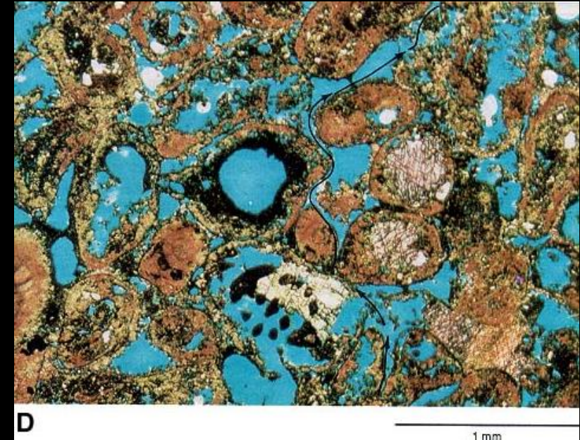
Limestone (black arrow = flow) Porous Permeable
