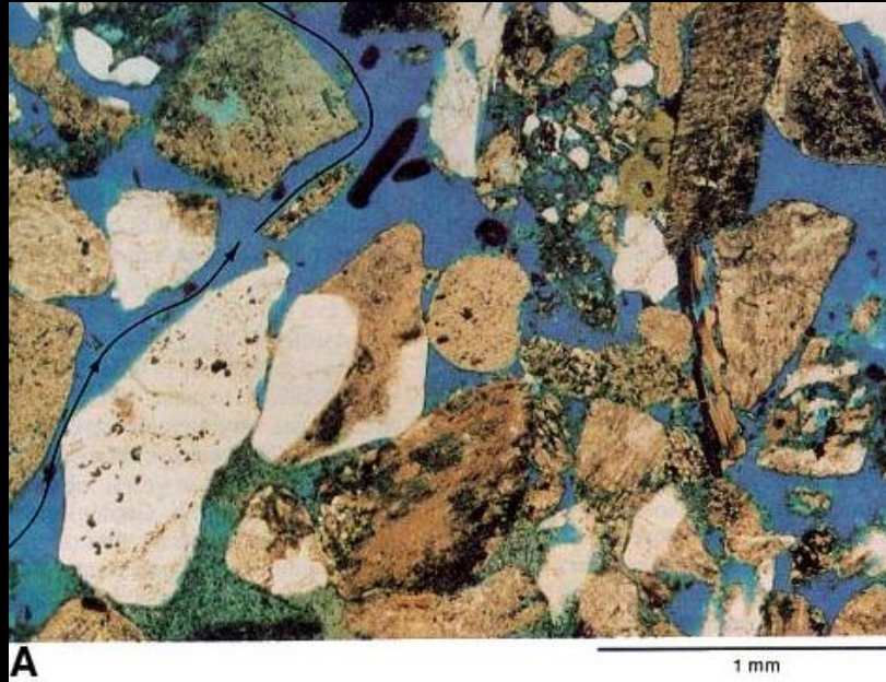
Sandstone (black arrow= flow) Porous Permeable
